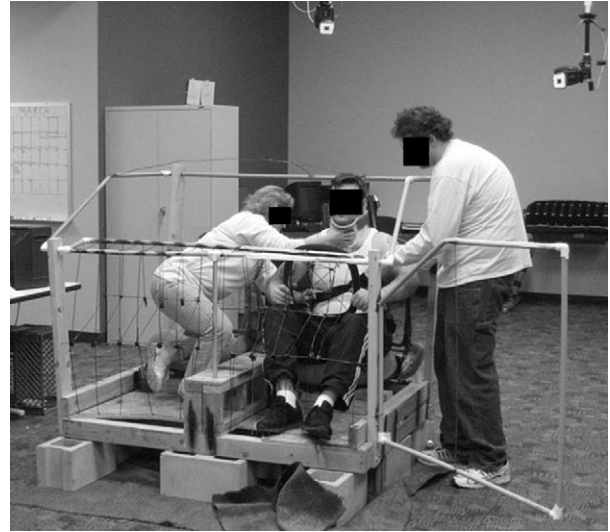
Figure 1. Application of the cervical collar by Emergency Medical Services personnel in the mock automobile. Visual monitoring cameras recording head and trunk movement of victim.
